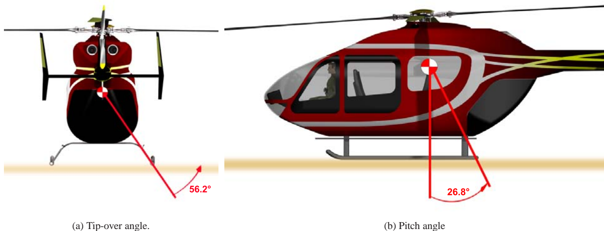
Figure 12.1: Center of gravity envelope of Griffin .
