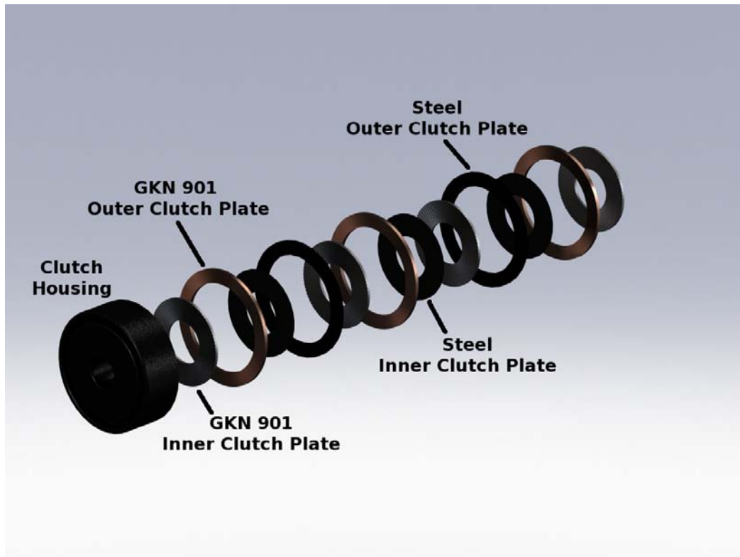
Figure 4.4: Wet clutch exploded view.
