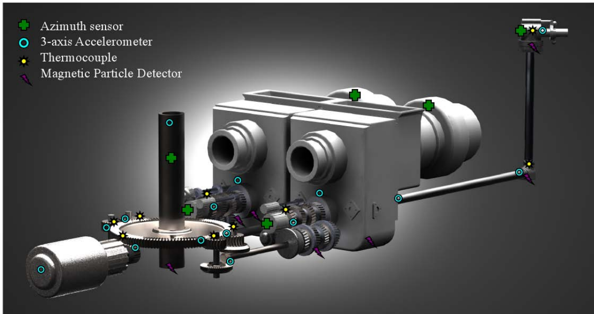
Figure 9.3: HUMS sensor configuration.
